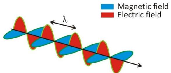
Figure 7: An electromagnetic wave is made of an oscillating electric field and, an oscillating magnetic field perpendicular to it, with the same periodicity. (Source: photonicswiki)
