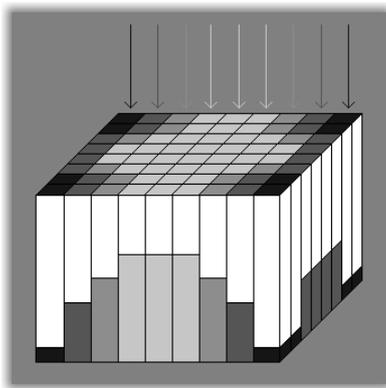
When a photon hits a square, an electron is released. The electrons are stored within the walls of a photosites.
