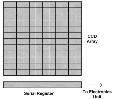
Figure 11: a 12x12 photosite CCD
