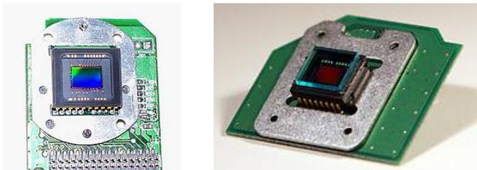
Figure 10 : CCDs from two different 2,1 pixel digital cameras (source: wikipedia)
