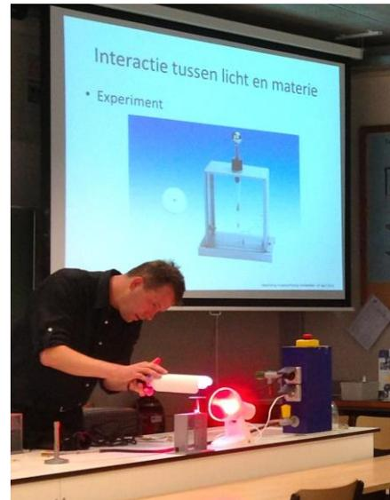
Figure 6: Belgian teacher Hans demonstrates the photoelectric effect with an electroscopes and a UV-C lamp.
